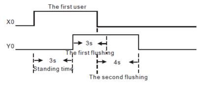
If the second user comes before the finishing of the 4 sec flushing, the flusher will finish the
