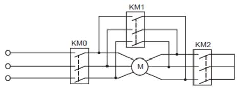
Reduced Voltage Starting Main Circuit
