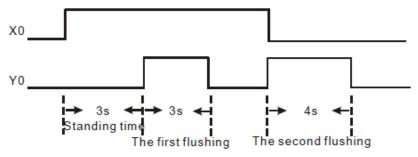
Stopping the first flushing and starting the second flushing if the first user leaves the urinal during the first flushing process.
